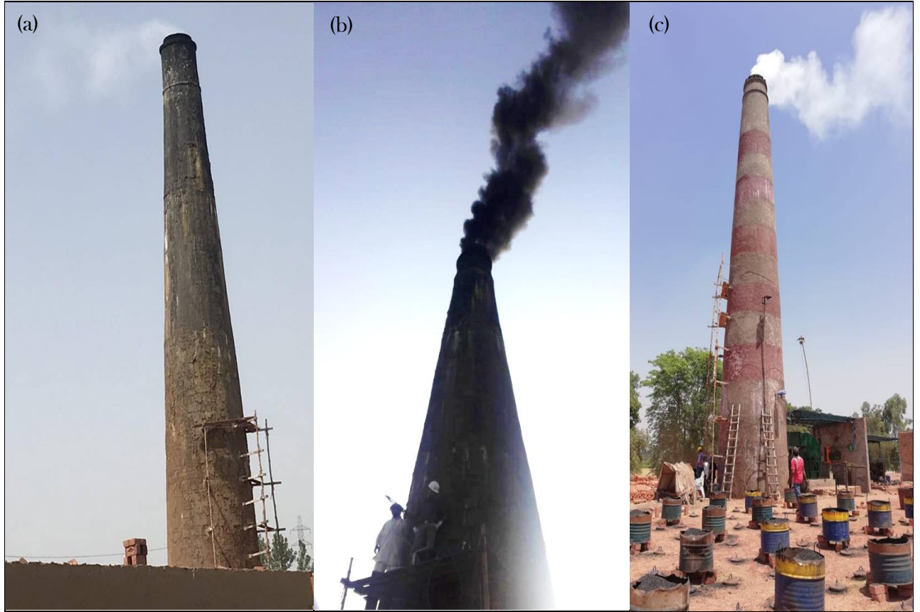
Figure 1: Stack emission sampling of: (a) BTK during non-feeding cycle; (b) BTK during feeding cycle; and (c) ZZK.
