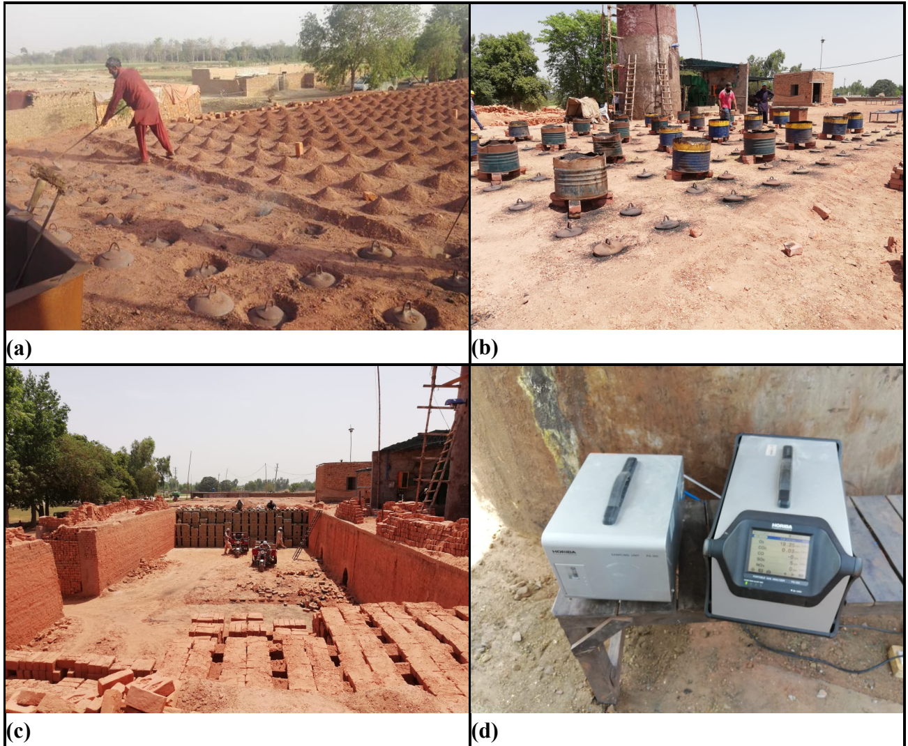
Figure A1: (a) Fuel feeding at the BTK, (b) Fuel feeding at the ZZK, (c) Stacked green and fired bricks at the ZZK, (d) Horbia PG-350E used for measuring stack gaseous emissions.
